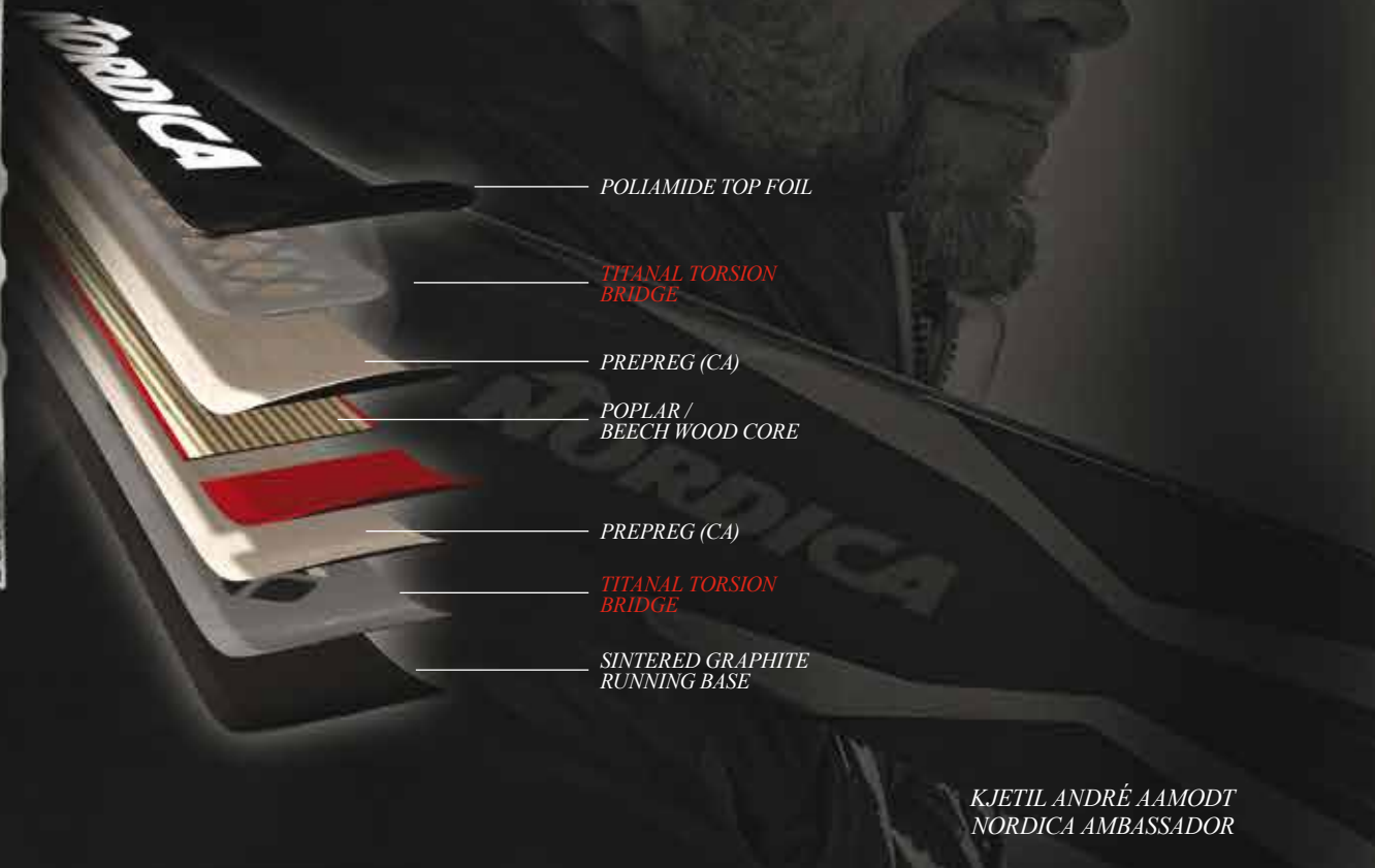
ENERGY 2 TITANIUM TORSION BRIDGE CONSTRUCTION
